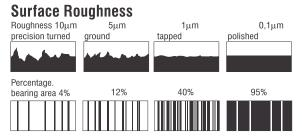
Lapped sliding face made out of different materials having the following average, arithmetic mean roughness values (Ra)
